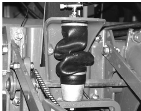
Improperly Rolled Air Spring
